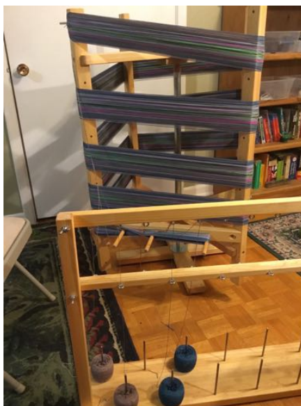
Vertical reel (2.5 m circumference) (could be table mounted) and thread holder
